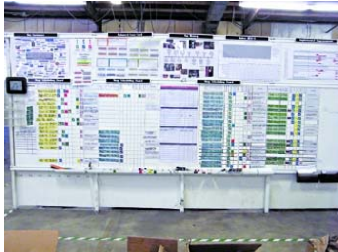
This one chart of Glastonbury-based Habco, which has boosted production efficiency through lean manufacturing, allows employees to monitor nearly all aspects of the business at any time.
